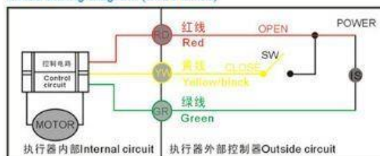
CR04(断电复位控制方式) CR04 Wiring diagram (power off return)
