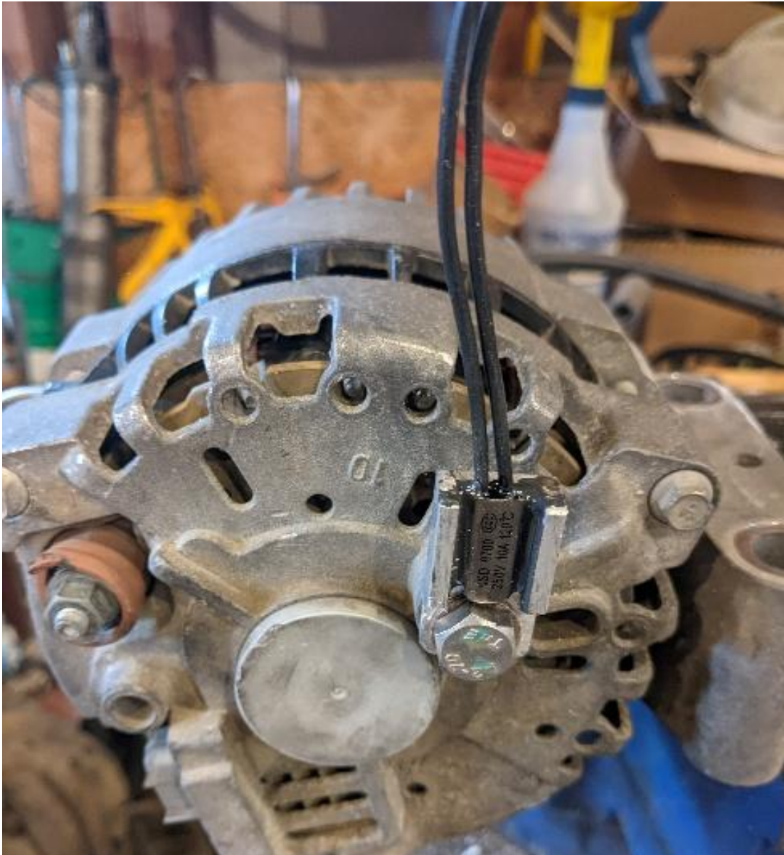
Figure 5: Thermal switch on an alternator
